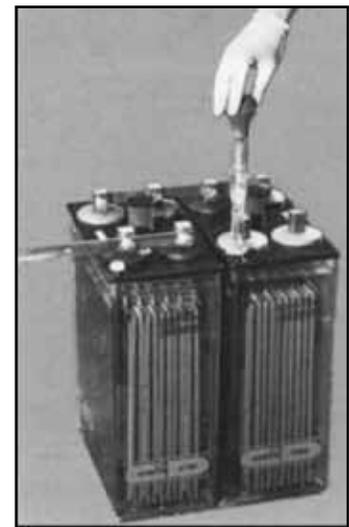
FIGURE 2.6.1 - Taking a hydrometer reading
