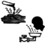
THIS BATTERY CONTAINS SULFURIC ACID, WHICH CAN CAUSE SEVERE BURNS. IN CASE OF SKIN CONTACT WITH ELECTROLYTE, REMOVE CONTAMINATED CLOTHING AND FLUSH AFFECTED AREAS THOROUGHLY WITH WATER. IF EYE CONTACT HAS OCCURRED, FLUSH FOR A MINIMUM OF 15 MINUTES WITH LARGE AMOUNTS OF RUNNING WATER AND SEEK IMMEDIATE MEDICAL ATTENTION.
