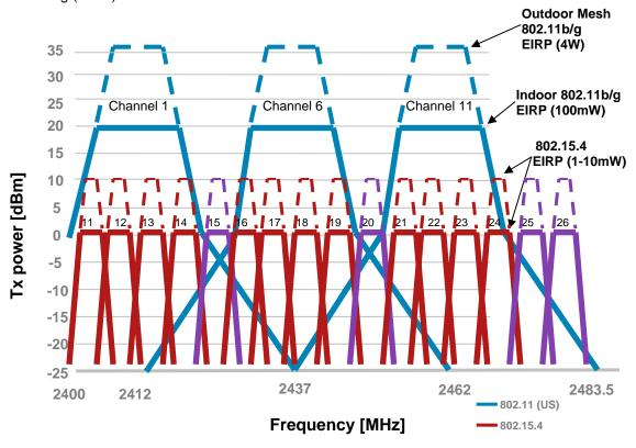
For overlapping channels, 802.11b/g radiated power is 10-100 times indoors than that of 802.15.4, and up to 4000 times for outdoor 802.11b/g mesh.
